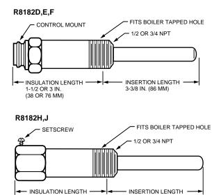
Fig. 3. Approximate immersion well dimensions.
