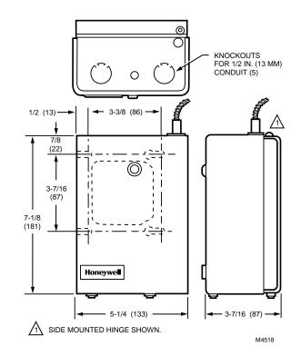
Fig. 2. R8182H,J installation dimensions in in. (mm).
