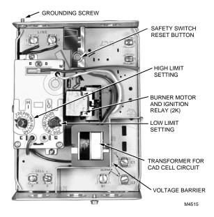
Fig. 6. Internal view of R8182F.
