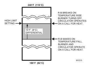
Fig. 19. R8182E,J Aquastat® limit switching.
