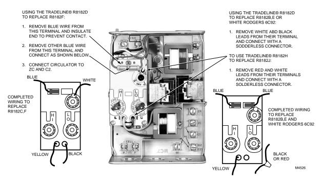
Fig. 10. Converting TRADELINE® R8182D,H to replace other controls.
