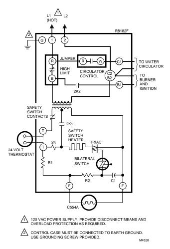
Fig. 13. R8182F internal schematic and wiring diagram.
