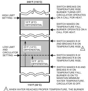
1 WHEN WATER REACHES PROPER TEMPERATURE, THE BURNER SHUTS OFF OR THE CIRCULATOR PUMP STARTS (WHEN CALLING FOR HEAT). M1523
