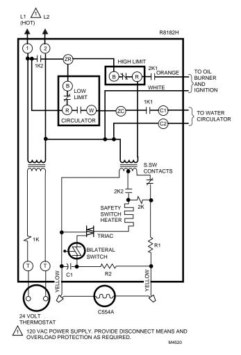
Fig. 14. R8182H internal schematic and wiring diagram.
