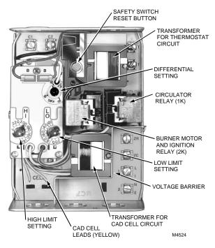
Fig. 7. Internal view of R8182H.
