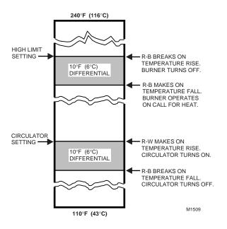
Fig. 20. R8182F Aquastat® limit switching.
