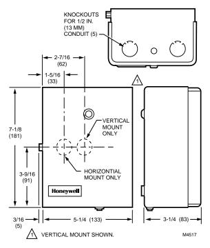
Fig. 1. R8182D,E,F installation dimensions in in. (mm).
