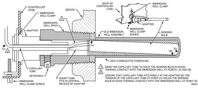
Fig. 9. Positioning the sensing bulb in the immersion well.
