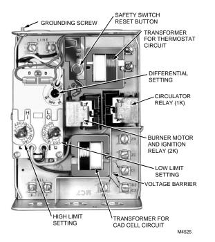
Fig. 4. Internal view of R8182D.
