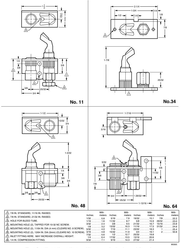
Fig. 4. Q314 No. 11, No. 34, No. 48 and No. 64 mounting brackets and dimensions.
