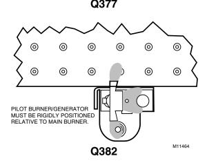
Fig. 17. Mount pilot burner on main burner (Q377 and Q382 shown).
