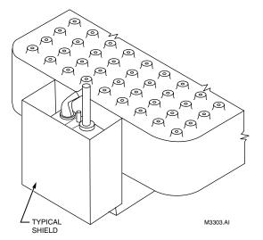
Fig. 25. Proper shielding of pilot flame (Q350 shown).
