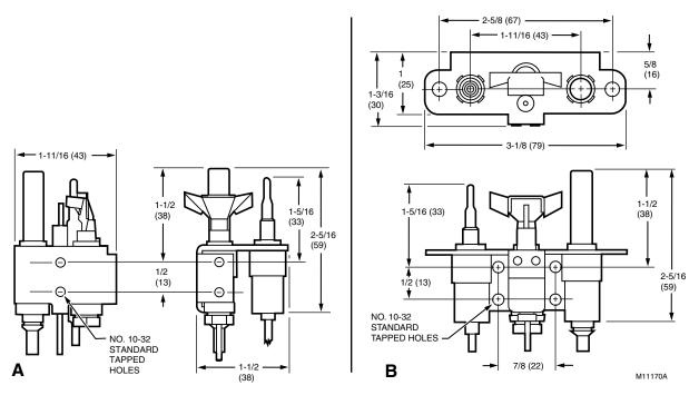
Fig. 15. Q382 mounting brackets and dimensions in in. (mm).
