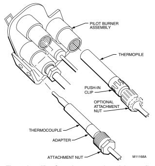
Fig. 21. Installing Q382 thermocouple and thermopile.
