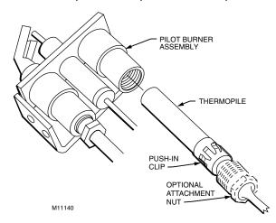
Fig. 20. Installing thermocouple or thermopile.
