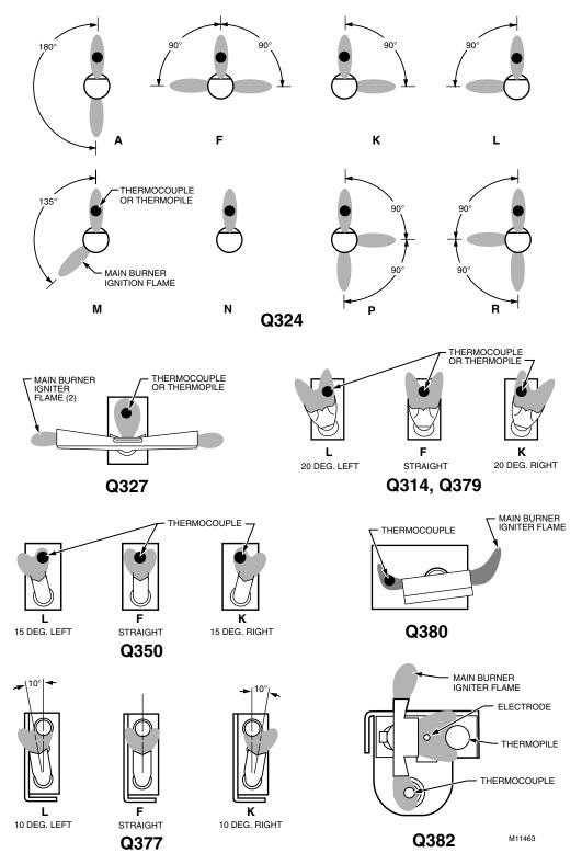
Fig. 2. Pilot Burner target and tip styles.
