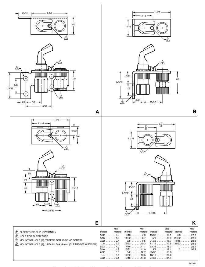
Fig. 3. Q314 A,B,E and K mounting brackets and dimensions.
