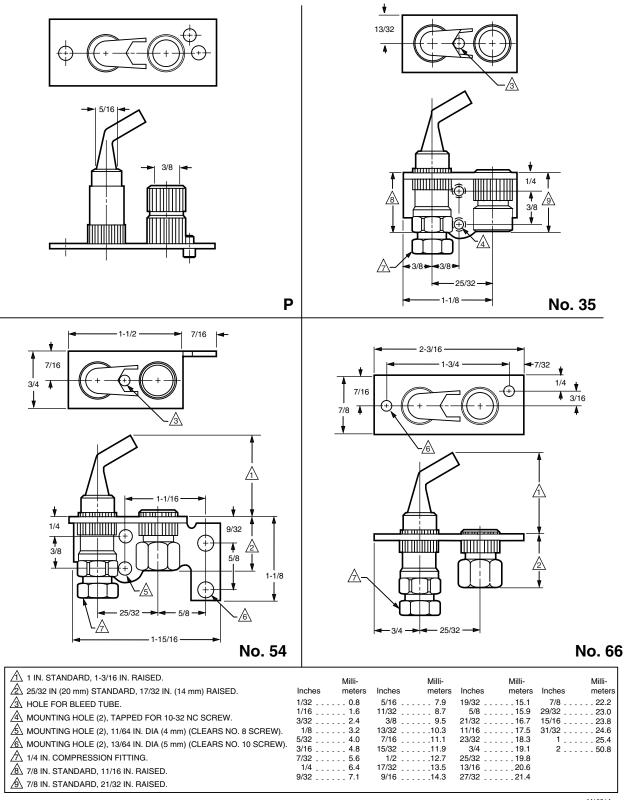
Fig. 10. Q350 P, No. 35, No. 54 and No. 66 mounting brackets and dimensions.
