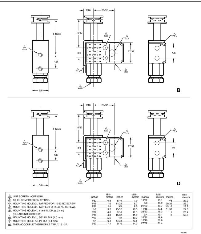
Fig. 5. Q324 B and D mounting brackets and dimensions.
