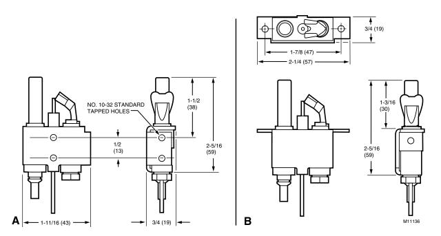
Fig. 13. Q379 mounting brackets and dimensions in in. (mm).
