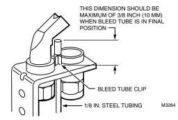
Fig. 22. Install bleed gas tubing.
