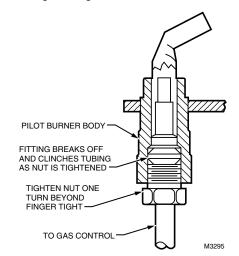
Fig. 19. Always use new compression fitting.
