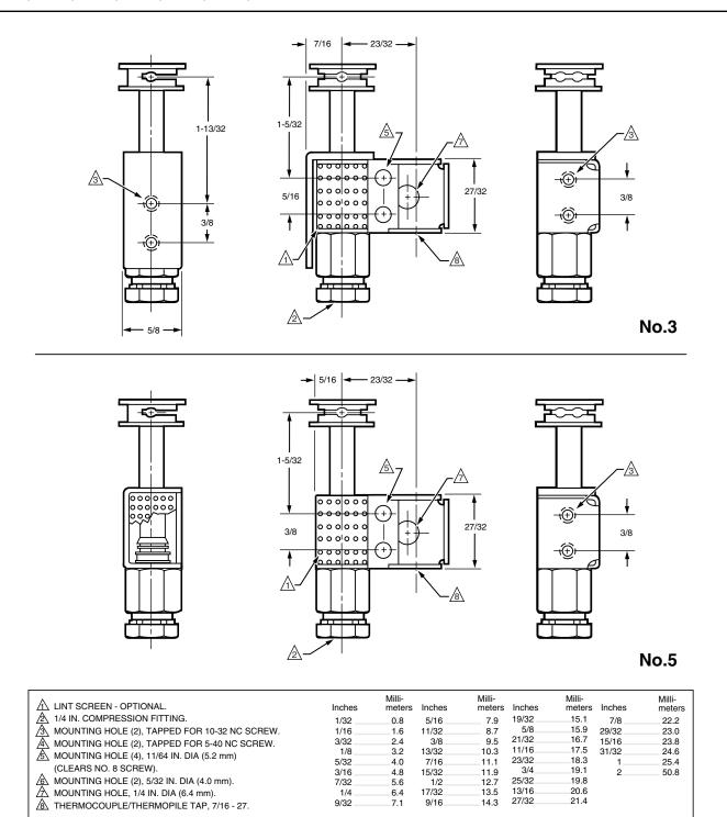
Fig. 6. Q324 No. 3 and No. 5 mounting brackets and dimensions.
