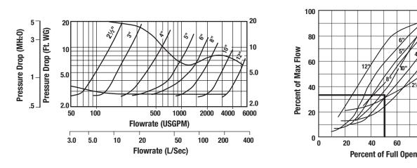
Series TDV Performance Curve with Valve in Full Open Position
