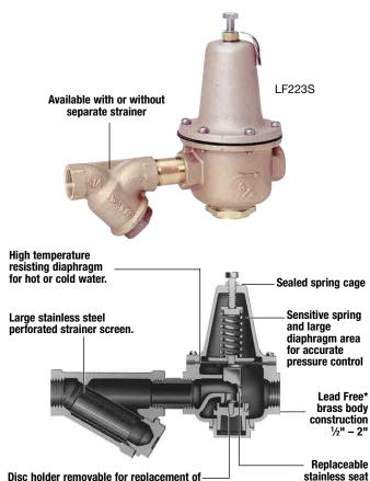
Disc holder removable for replacement of disc without dismantling the valve no special tools required.
