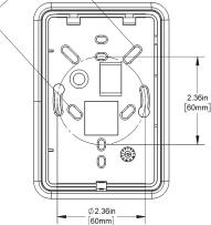
Fig. 4: 60mm mounting base dimensions
